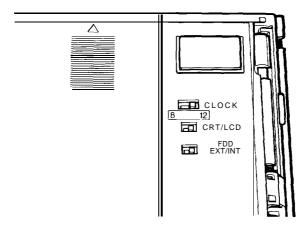
The CLOCK switch has two positions. The left position is 8 MHz; the right position is 12 MHz.
